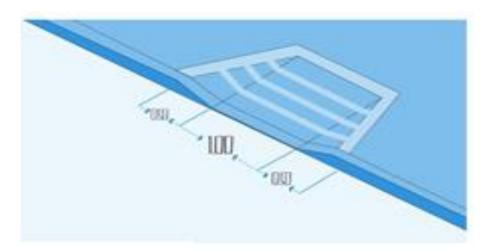
In addition to the use of non-slip flooring, the minimum length and width must follow the standard in the table below:
